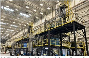
NOVONIX Generation 3 Continuous Induction Furnace Systems
