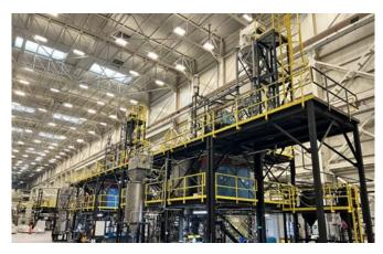
Two Generation 3 Furnace systems and milling equipment installed in NOVONIX's Riverside facility
