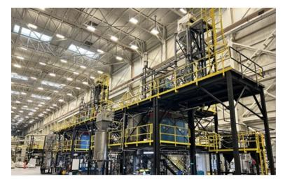
NOVONIX Generation 3 Continuous Induction Furnace Systems
