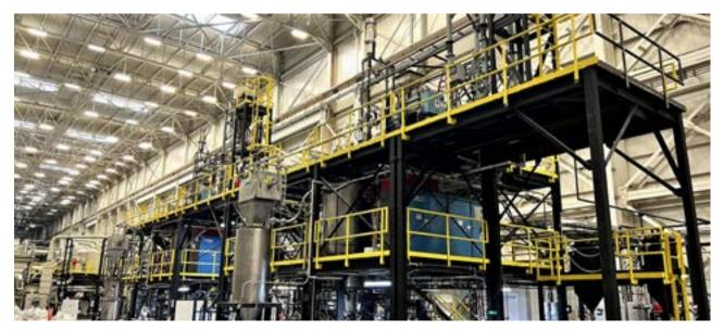
Generation 3 Furnace systems and milling equipment installed in NOVONIX's Riverside facility
