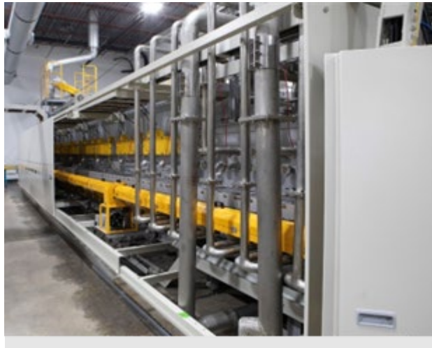
NOVONIX 13.5 m long pilot roller hearth kiln (RHK).
