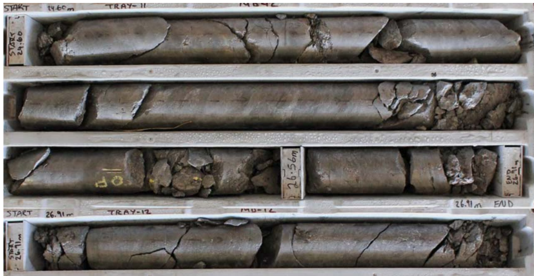
Image: HQ diamond core – Drillhole MD-12 - Central Zone of the Mount Dromedary December 2015.
