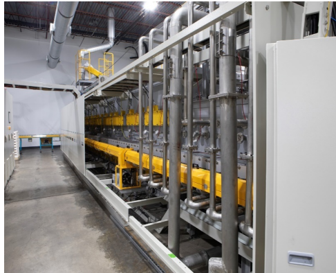
NOVONIX 13.5 m long pilot roller hearth kiln (RHK) with partial insulating panels removed displaying assortment of gas handling plumbing, banks of resistance heaters (yellow rectangles, top), and roller conveyance mechanism (yellow, middle).
