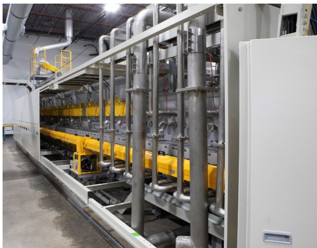
NOVONIX 13.5 m long pilot roller hearth kiln (RHK).
