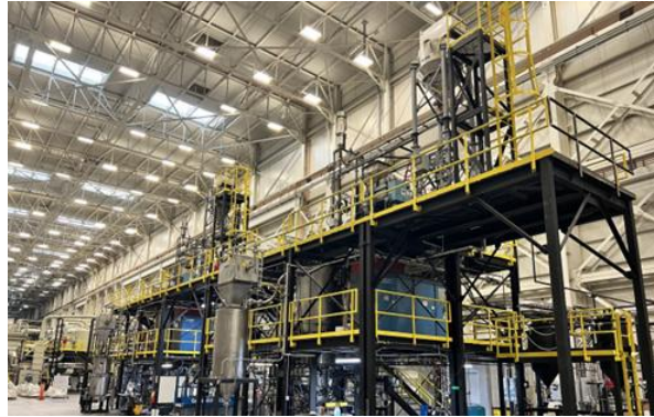
Two Generation 3 Furnace systems and milling equipment installed in NOVONIX's Riverside facility
