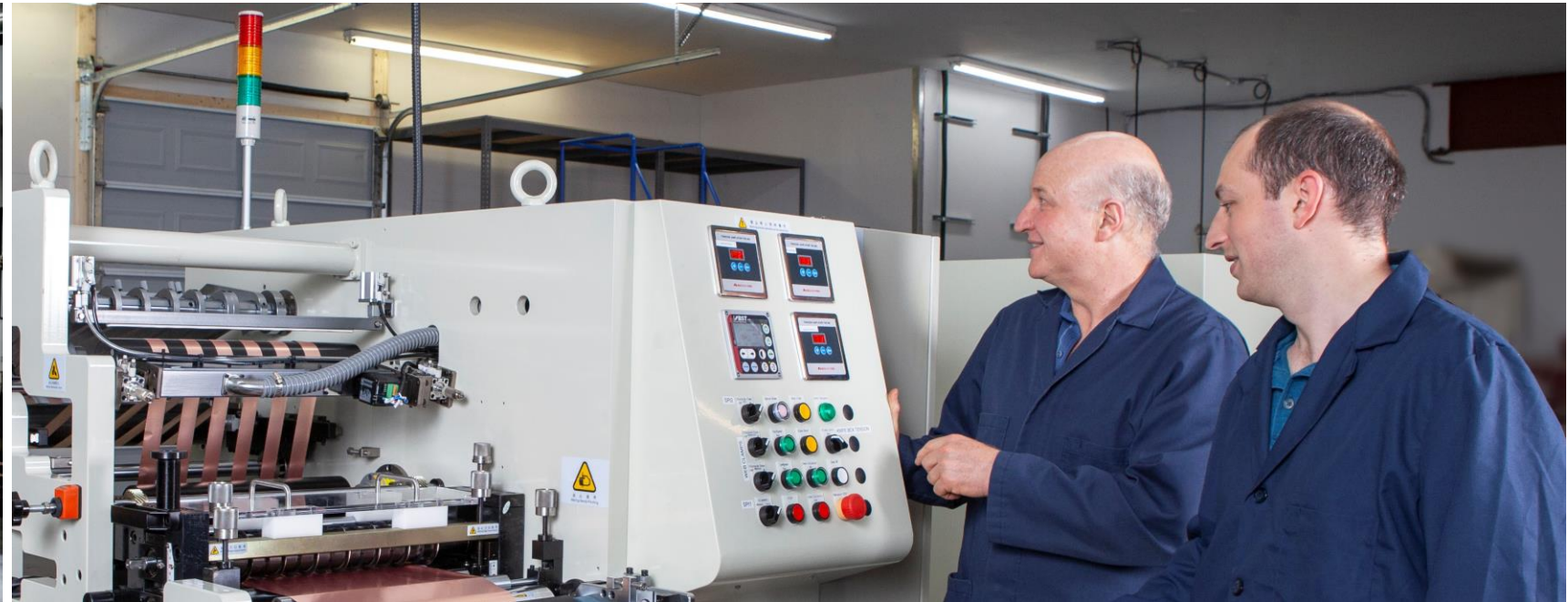
Photo: Professor Jeff Dahn of Dalhousie University with Dr Chris Burns NOVONIX COO inspecting the electrode slitting operation at the NOVONIX battery cell manufacturing facility
