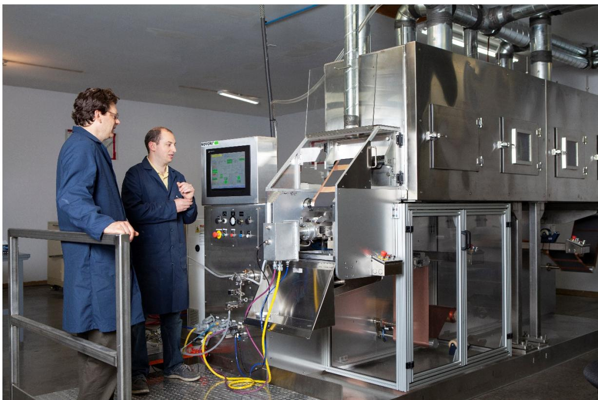
*Photo: Professor Mark Obrovac of Dalhousie University and Dr Chris Burns COO NOVONIX inspecting the electrode coating line at the NOVONIX battery cell manufacturing facility*
